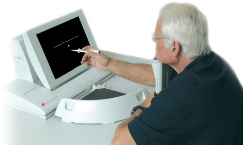
Figure 2. The Foresee Preferential Hyperacuity Perimeter (Foresee PHP™). The patient is positioned on a chin rest and directs their gaze at a central fixation target. A stylus is used to record on a touchscreen video monitor the location of the perceived distortion of a dotted line stimulus. (Image courtesy of Notal Vision, Tel Aviv, Israel: http://www.notalvision.com ).
